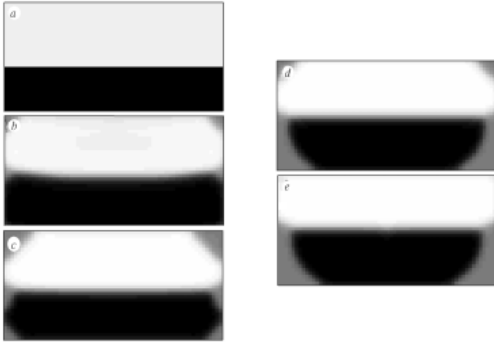
Fig. 4. Problem 2. Binodal disintegration of the mixture into two phases (A and C) in the presence of the third phase B (phase A, white color, B, black, and C, gray): a) t = 0 , b) 7.2, c) 80.5, d) 706.9, and e) 2120.7 min.
